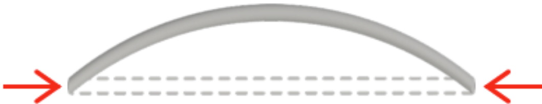
Figure 2.4: Global buckling failure mode of a CHS member.
