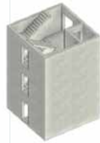
1 Core / Bracing System
